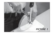
Picture 1). Exert downward pressure on the nut just until it loosens.
