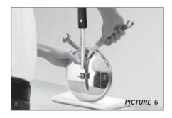
will be facing you. With the right hand, position the second spanner around the nut under the lid handle bar at an upward angle and exert downward pressure on the spanner (see **Picture 6**). Tighten the nut securely by repeating the downward strokes of the spanner until the nut stops moving.
