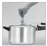
The pressure regulator has a spring mechanism which holds the pressure regulator on to the steam vent and is strong enough to prevent it from falling off should the lid be inverted.
