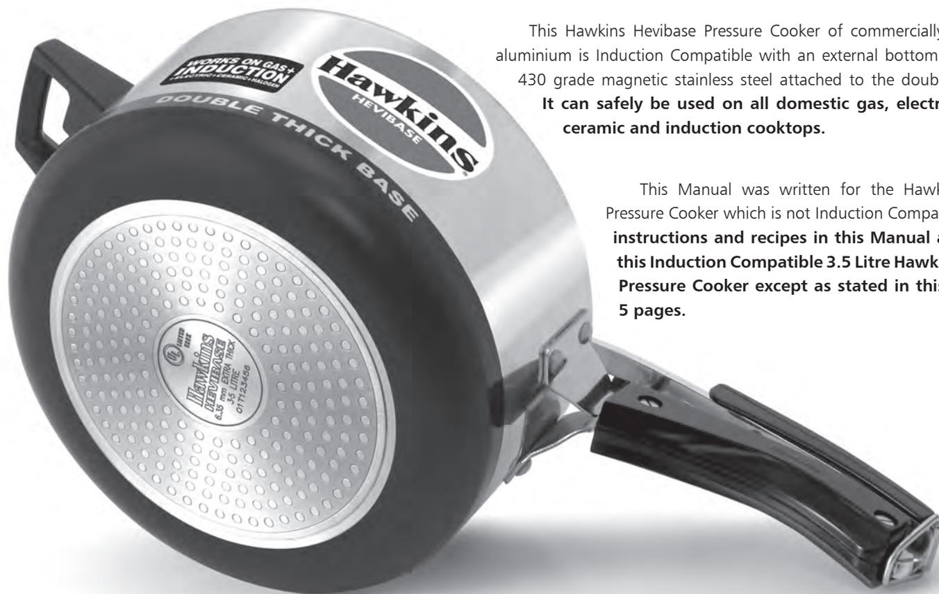
This Hawkins Hevibase Pressure Cooker of commercially pure, virgin aluminium is Induction Compatible with an external bottom plate of AISI 430 grade magnetic stainless steel attached to the double thick base.
