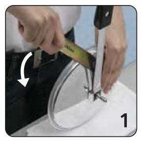
Hold lid as shown, on soft surface or folded cloth. Place spanner around nut on top of lid. Turn downward just until it loosens. If too tight, soak lid in hot water for 10 minutes.
