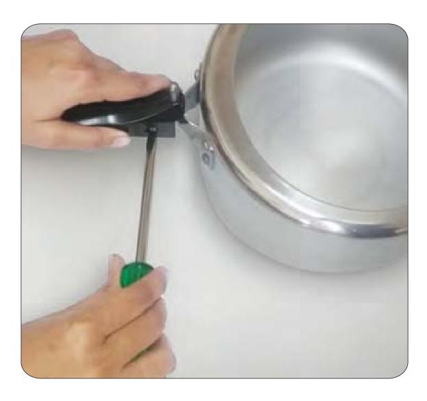
Unscrew existing handle. Screw on the replacement Body Handle. For best results, use a 6 mm tip screwdriver (not supplied in the Kit).
