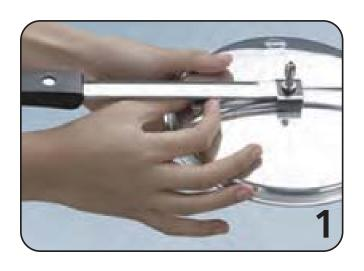
Clean around the lid hole where the safety valve will sit. Unscrew new nut, keep to one side. Push retainer with silicone washer
