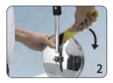
Hold lid vertically as shown (with top of lid facing you). Position spanner around nut at an upward angle and exert downward
