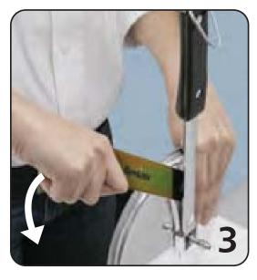
Now re-apply spanner on nut and turn. Remove, re-apply spanner at a higher angle, and repeat downward pressure, until nut can be unscrewed with fingers. Remove and
